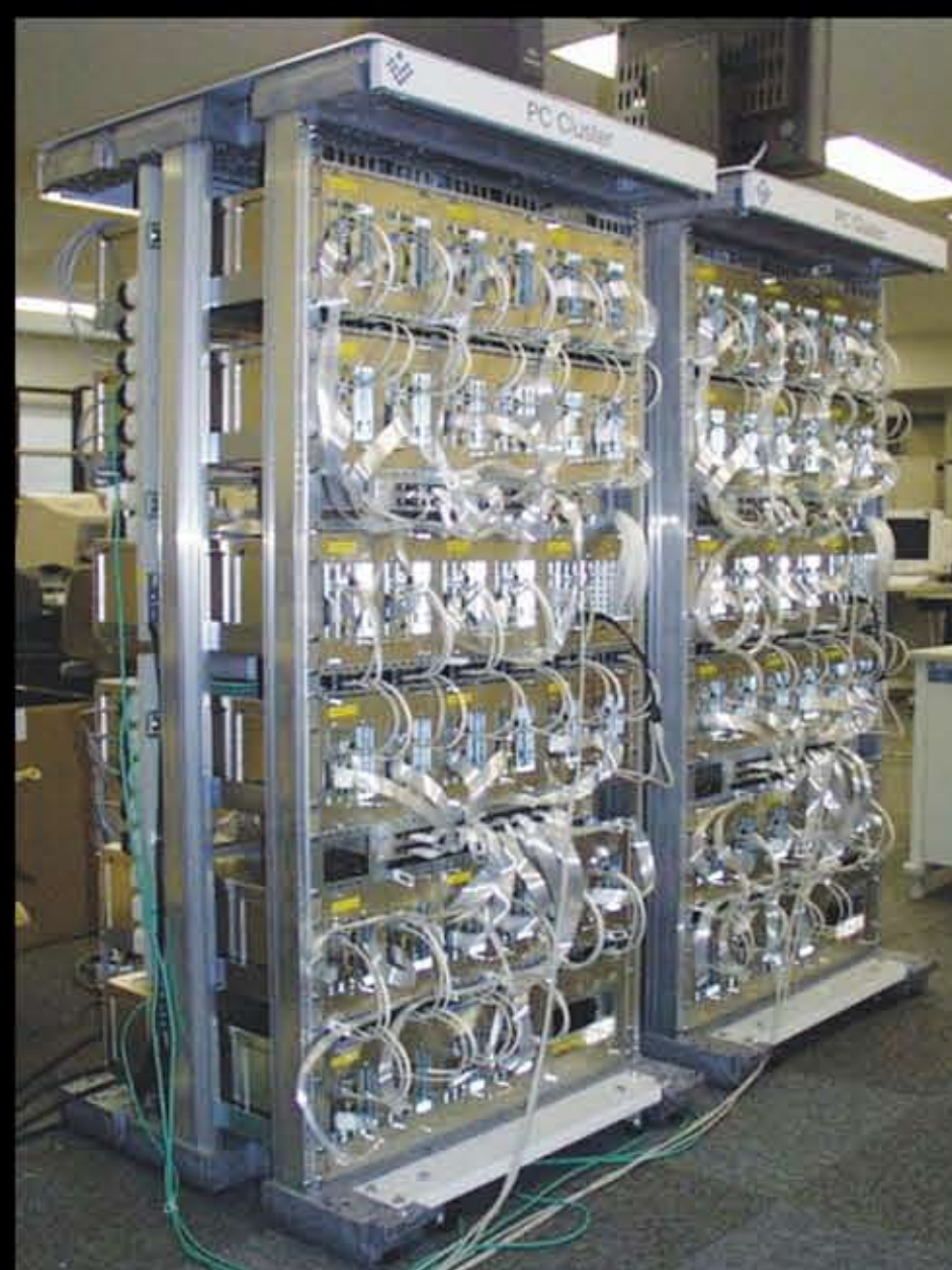
A 64 node PC-based Beowulf cluster
