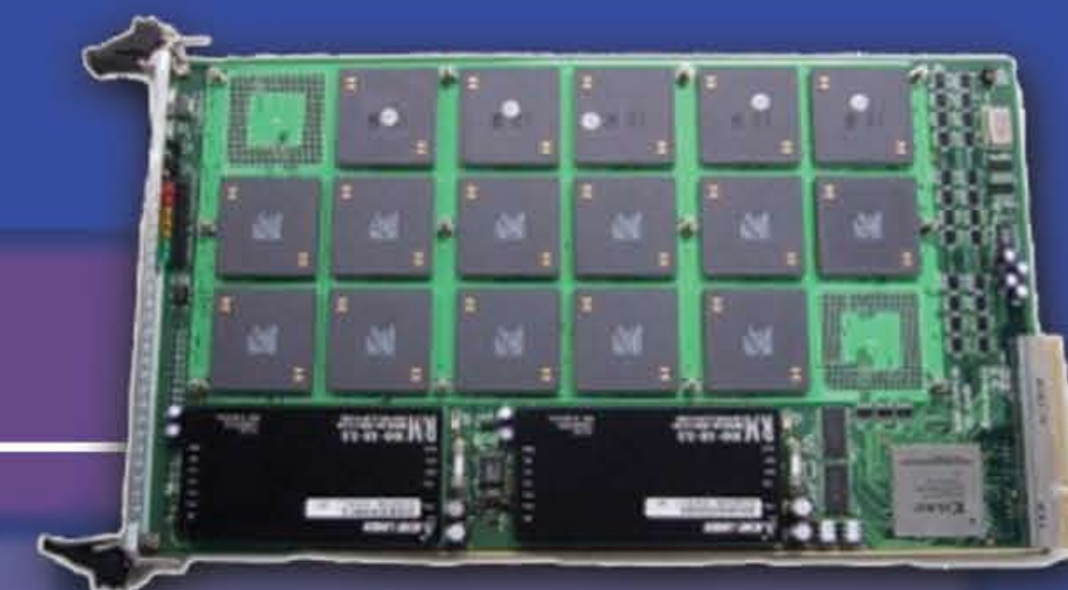
A WINE-2 system board
