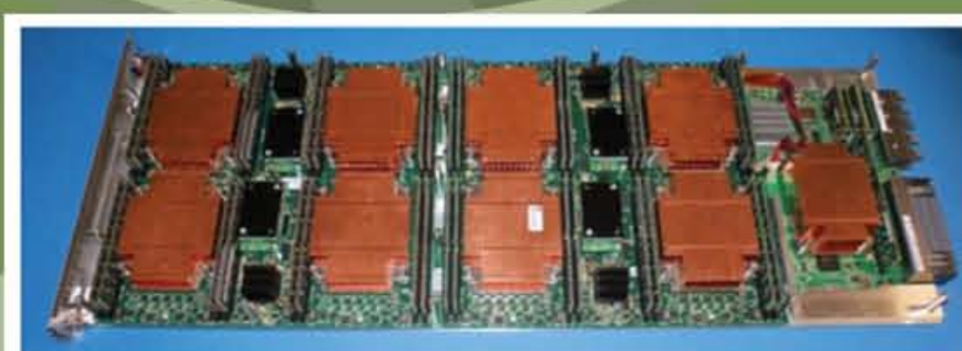
Figure 1. A Cascade blade which consists of 8 Xeon sockets, organized as 4 dual-socket nodes, and a single Aries ASIC.
